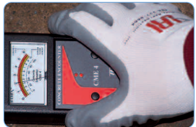
URI personnel testing the level of moisture in concrete. After a water damage, make sure to hire a qualified flooring expert before installing new floor covering.
